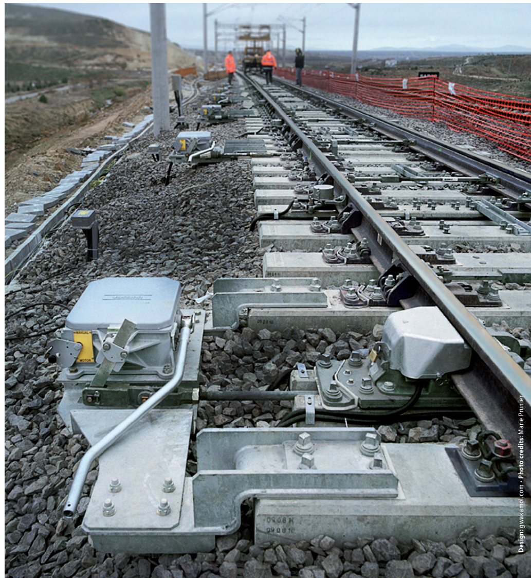
Multiple drive integrated into a 1/46 turnout – High Speed Line, Turkey
