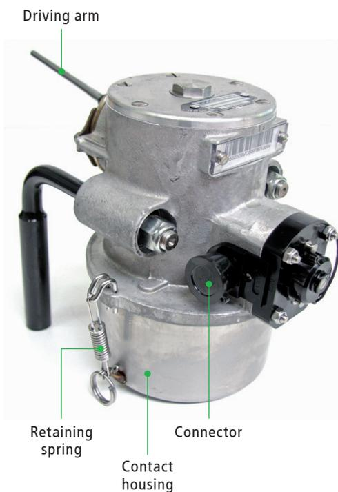
Detection is activated by the lowering of a driving arm pushed by the vehicle's passage. Both running directions can be detected.
