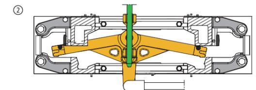
The movement of the drive rod will cause the rotation of the square and thus unlock the left-hand square head and disengage the right-hand square head from the wedging chamber.
