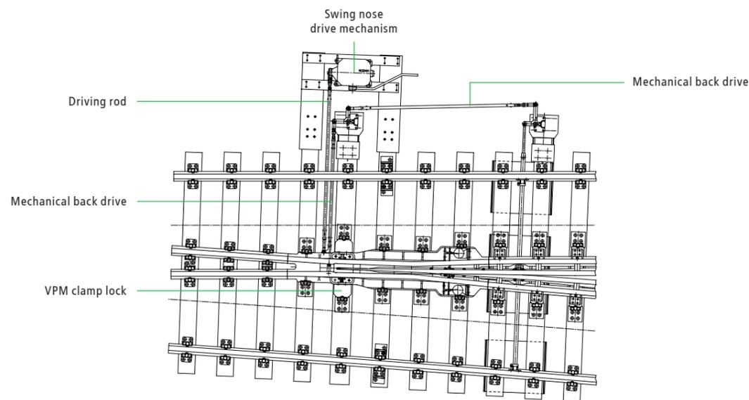
Endorsed by the most demanding networks, the swing nose clamp lock (VPM) meets the NF F 52-163 and NF F 52-164 safety standards. The UIC recommends it for high-speed lines (see UIC 734R) and the SNCF requires it on TGV (French high-speed rail network) lines (see NF 52-151).
