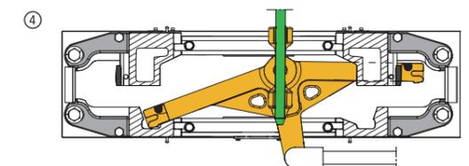
The movement of the drive rod will cause the rotation of the square and lock the right-hand square head and engage the left-hand square head into the wedging chamber.
