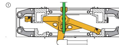
The VPM configuration is as follows: the swing nose is locked by the left-hand square head and wedged by the right-hand square.
