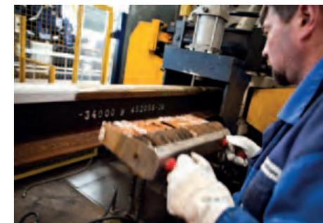
Numerical identification for tracking each weld joint
