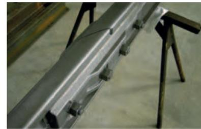
Completely glued angular joint IVB 30°
