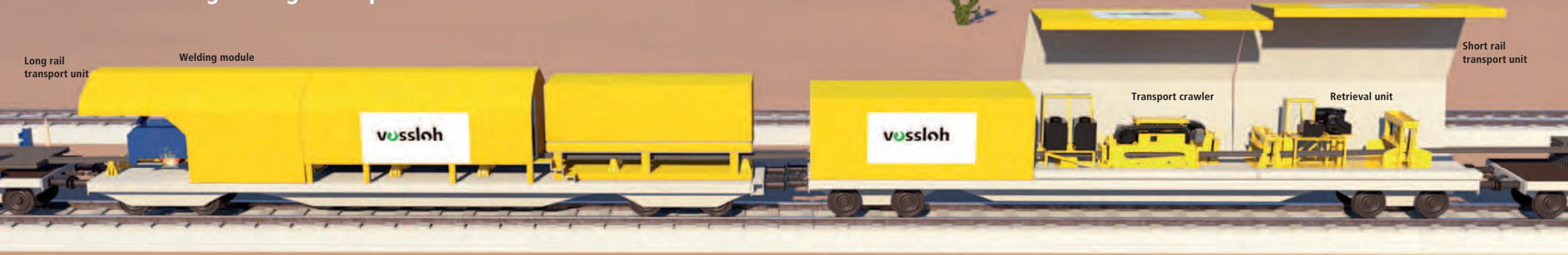
Short rails welded into long rails are pushed onto the transport unit, where the fine grinding takes place after cooling.
