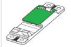
Slide chair with resilient fastening and sliding table without lubrication
